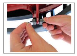
Lock the hood into place by fitting a hinge pin through the firebox flanges and the hood hinge arms on each side. Fix the hinge pin by inserting "R" clip through the end of each pin.
